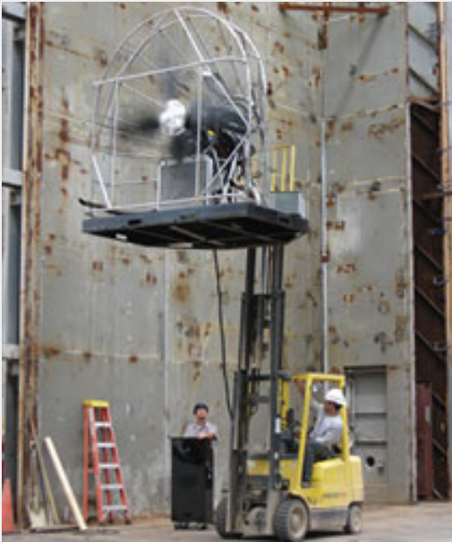
Photo 4: Portable Dynamic Wind Generator for Field Dynamic Water Testing
