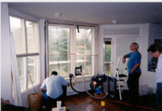
Photo 2: ASTM E 1105 Test Conducted in Accordance w/ AAMA 502-08 Voluntary Specification
