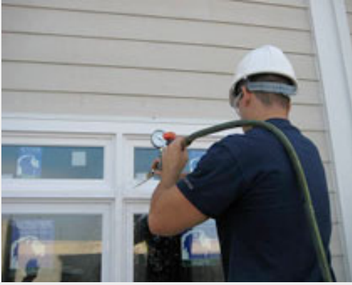
Photo 3: AAMA 501.2 Test on Fixed Transom Window
